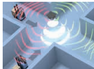
Two vehicles simultaneously: slow flashing will be triggered
