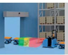
The precision and accuracy of the 3D sensor technology detects trailers of tow trucks and reliably prevents rear-end collisions.
